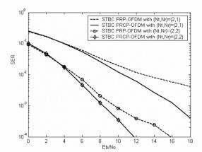
**Figure 3** Comparison of SER for ST-BC PRP-OFDM and ST-BC CS-PRP-OFDM with orthogonal cyclic sequence.
