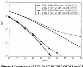
Figure 4 Comparison of SER for ST-BC PRP-OFDM and CS-PRP - OFDM with orthogonal cyclic sequence.
