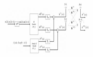
Figure 1 Block diagram of the ST-BC MIMO PRP-OFDM modulator
